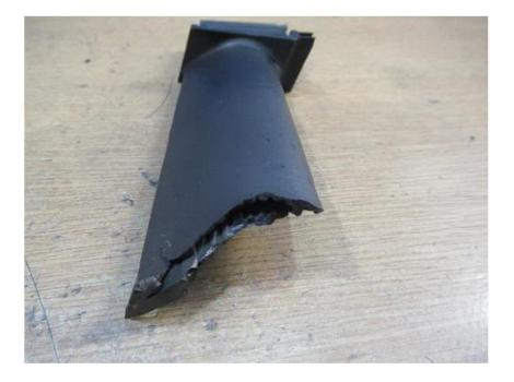
Figure 2: Failed High Pressure Turbine Blade
