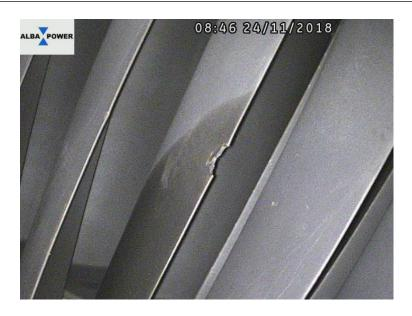
Figure 3: Low Pressure Turbine Blade Impact Damage
