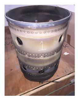
Figure 4: Exterior of Failed Combustion Can From Engine 202205
